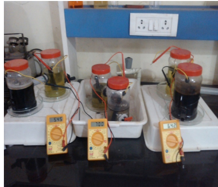
Plate2: Other MFCs set up used during work at laboratory
